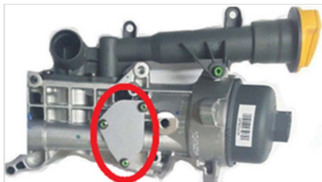
Cooling radiator for private oil from the heat exchanger and equipped with a closing plate
